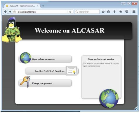
Click on the small cranted wheel at the bottom right in order to connect to the <u>A</u>LCASAR <u>C</u>ontrol <u>C</u>enter (ACC). You must authenticate you with the first account created during the installation process ( $\S$ 2.3 – P10 of this document).
